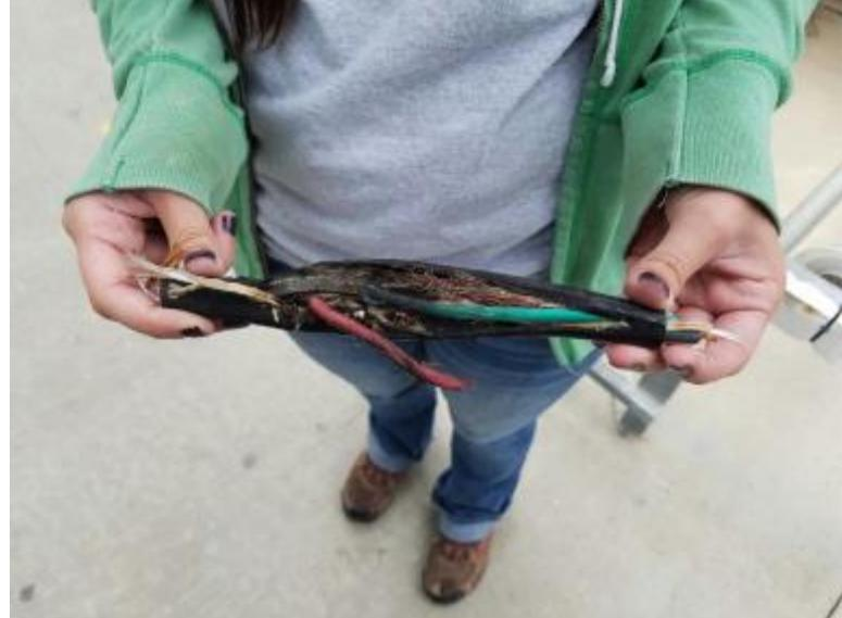
Picture of a time that I forgot to unplug the sprayer when moving to the next house and I stretched the cord so far it ripped open and sparked. But they fixed it!
